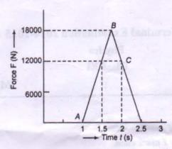
The figure above shows force time graph for a base ball struck by a bat. Determine the
