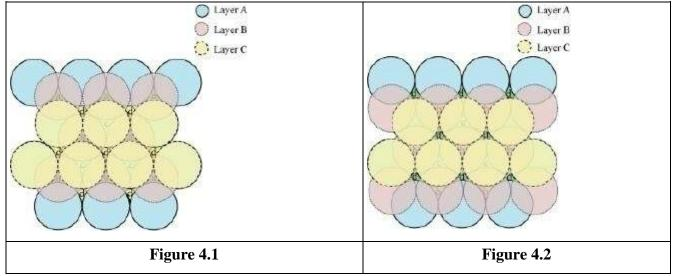
Case 2: When the third layer (layer C) is placed over layer B in such a manner that the spheres of layer C occupy the octahedral voids d.
