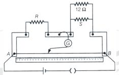
47. In a meter bridge, the null point is found at a distance of 60 cm from A. If a resistance of 5Ω is connected in series with S, the null point occurs at 50.0 cm from A. Determine the values of R and S. [Delhi 2010]
