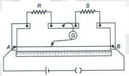
**48.** In a meter bridge, the null point is found at a distance of  $l_1$  cm from A. If a resistance of X is connected in parallel with S, the null point occurs at a distance  $l_2$  cm from A. Obtain the formula for X in terms of  $l_1$ ,  $l_2$  and S.
