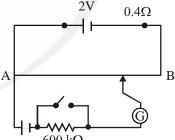
86. Figure shows a potentiometer circuit for comparison of two resistances. The balance point with a standard resistor  $R = 10.0 \Omega$  is found to be 58.3 cm, while that with the unknown resistance X is 68.5 cm. Determine the value of X. What might your do if you failed to find a balance point with the given cell of emf  $\epsilon$ ?
