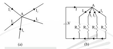
Consider the case of a few conductors meeting at a point A as in figure (a). Some conductors have current leading to point A. Whereas some have currents leading away from point A. Assuming the incoming currents to be positive and the outgoing currents negative, we have
