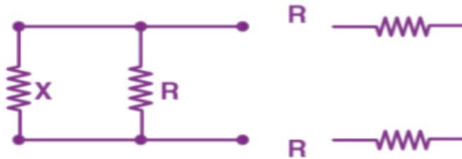
The equivalent resistance of this network is  $R' = R + (\text{equivalent resistance when } X \text{ and } R \text{ are parallel}) + R$
