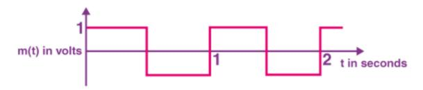
The carrier wave is given by  $c(t)=2\sin(8\pi t)$  volts.
