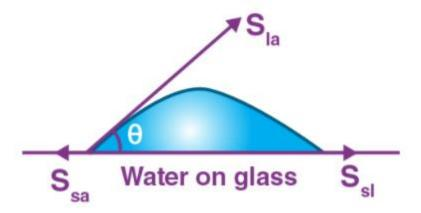
In the diagram  $S_{sl}$ ,  $S_{la}$  and  $S_{sa}$ , are the respective interfacial tensions between the liquid-solid, liquid-air, and solid-air interfaces. At the line of contact, the surface forces between the three media are in equilibrium, i.e.,
