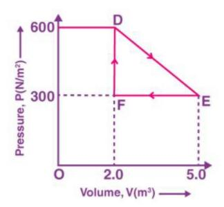
Its volume is then reduced to the original value from E to F by an isobaric process. Calculate the total work done by the gas from D to E to F
