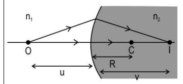
For a plane refracting surface, the curved surface formula gets modified as:  $n_2/v = n_1/u \dots (2)$
