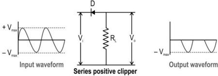
Similarly, just by reversing the diode, only the negative half cycles are removed. This is Series Negative Clipper circuit.
