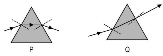
Select the suitable surrounding mediums from the given table of refractive indices here for each of the above refractions through the prisms P and Q. Give reason for the choice of the mediums.
