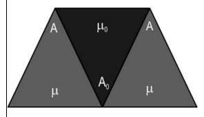
Prove that for a net deviation produced in the light ray to be zero,  $\mu = \mu_0$  in the given combination.
