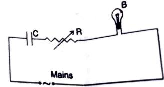
A dielectric slab is introduced between the plates of the sana
